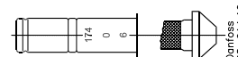
Orifice assembly and filter for flare x flare version for T2 and TE2
